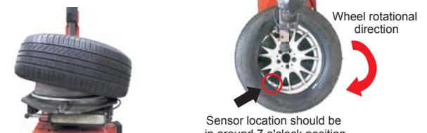
Sensor location should be in around 7 o'clock position
